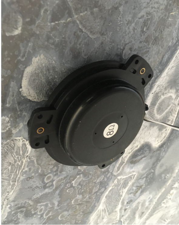
Audio transducer and contact microphone (Brian House)
