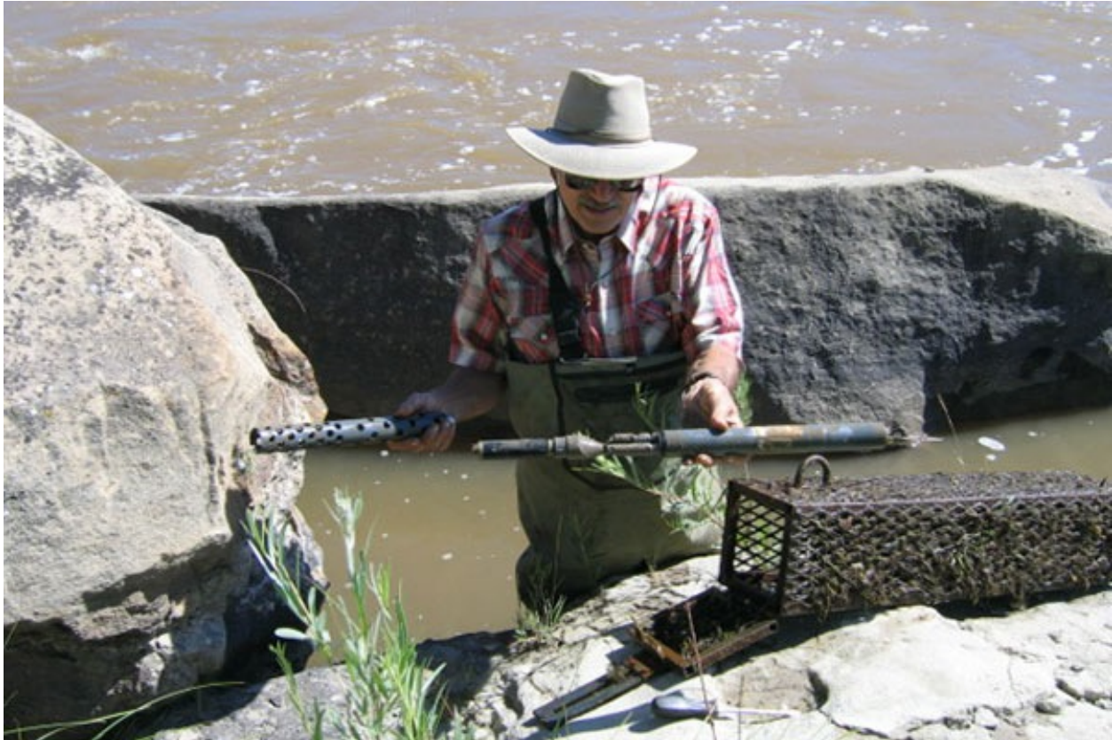
Kirk Lashmett of the SUIT Water Quality Program inspecting a sonde (SUIT Water Quality Program, used with permission)
